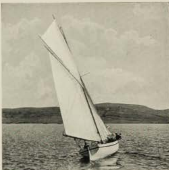
From a Photo. By a Naval Officer. A 36-ft. PINNACE, CUTTER RIGGED.
