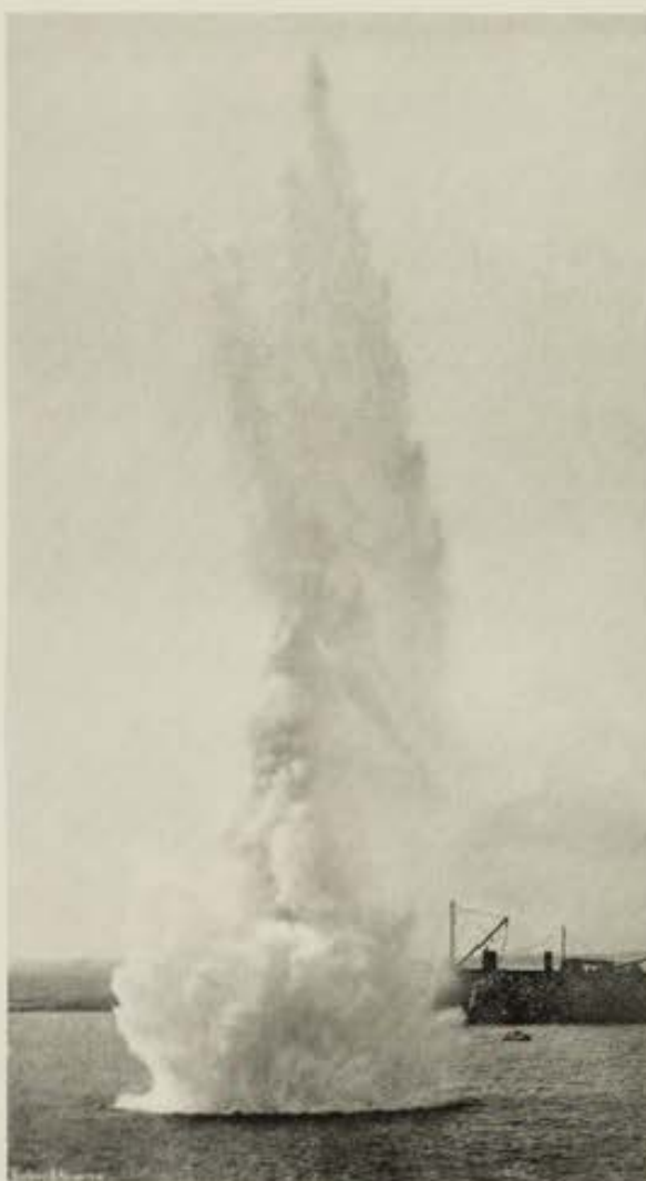
EXPLOSION OF A MINE CONTAINING 500-LB. OF GUN-COTTON.
