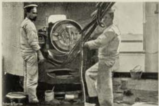
ARMOURERS STRIPPING A 6-in. B.L. GUN.
